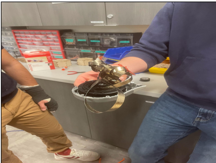
Figure 1.5: Torsion Spring and Spool
