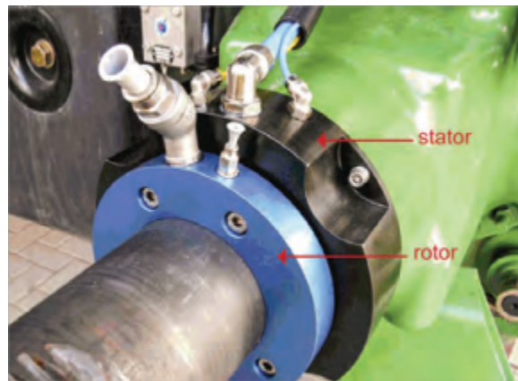
Figure 5: Air transmission unit for a bar axle [20].
