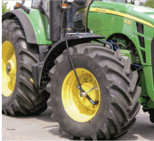
Figure 4: John Deere tractor equipped with CTIS [20].
